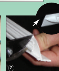
2 Mitre cut - snip inner leg as shown
